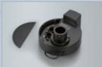
Fluorescence barrier filter positions (8 positions—using 25mm filters) can be changed at a high speed of 0.15 sec. per position.
